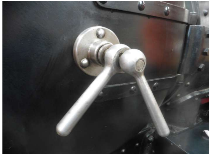
I wire-woolled and cleaned the sliding bars, and the smokebox door handles
