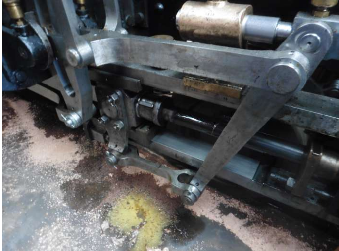
I wire-woolled and cleaned the sliding bars, and the smokebox door handles
