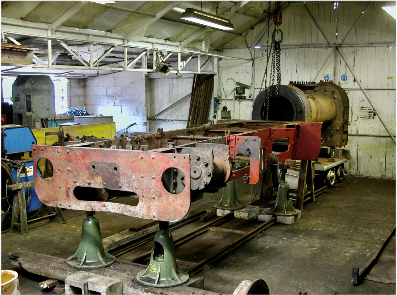
The Edward Sholto frames and boiler in the bottom shop
