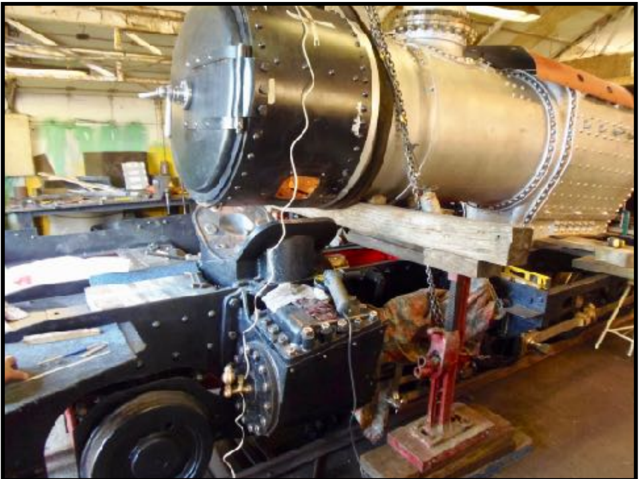
Smoke box lifted to allow the grinding of the saddle
