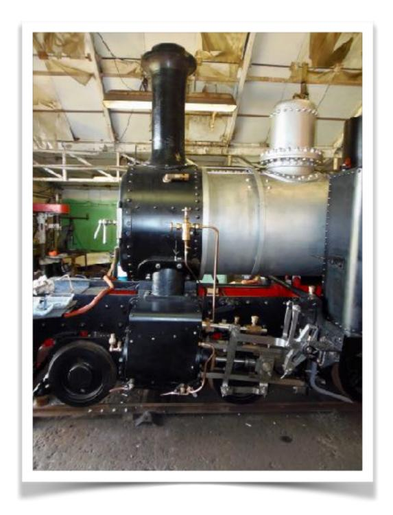
The drain cocks are now piped up, fitted and working, as are the Roscoe's
